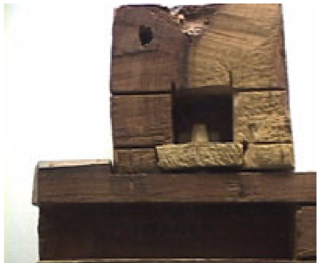
Figure LSS+102. Examples of different approaches to the original Egyptian pin tumbler design. These locks have been gathered from different countries, and demonstrate that the idea of using pins or pegs to secure a moving bolt or locking piece was not unique to any one society, although the Egyptians are credited with the initial concept. These exhibits are on display at the Science Museum in London.
