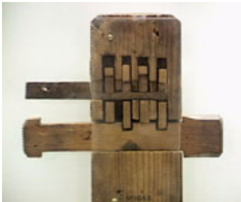
Figure LSS+102. Examples of different approaches to the original Egyptian pin tumbler design. These locks have been gathered from different countries, and demonstrate that the idea of using pins or pegs to secure a moving bolt or locking piece was not unique to any one society, although the Egyptians are credited with the initial concept. These exhibits are on display at the Science Museum in London.
