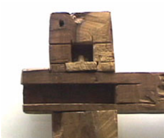
Figure LSS+102. Examples of different approaches to the original Egyptian pin tumbler design. These locks have been gathered from different countries, and demonstrate that the idea of using pins or pegs to secure a moving bolt or locking piece was not unique to any one society, although the Egyptians are credited with the initial concept. These exhibits are on display at the Science Museum in London.
