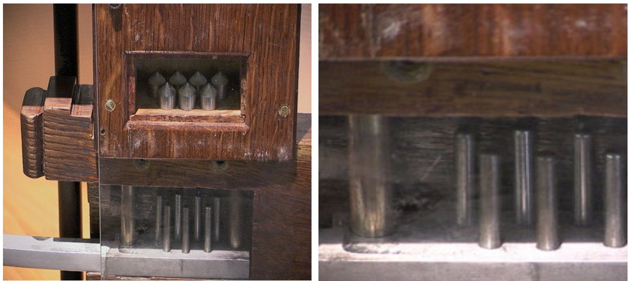
Figure LSS+101. A mock-up of the original Egyptian lock, produced by the British Museum, London. This replica shows the interaction of the protruding pegs with the internal pins.
